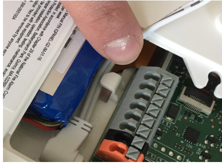
Route the wire behind the retainer clip
